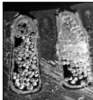
Poor slot fill
